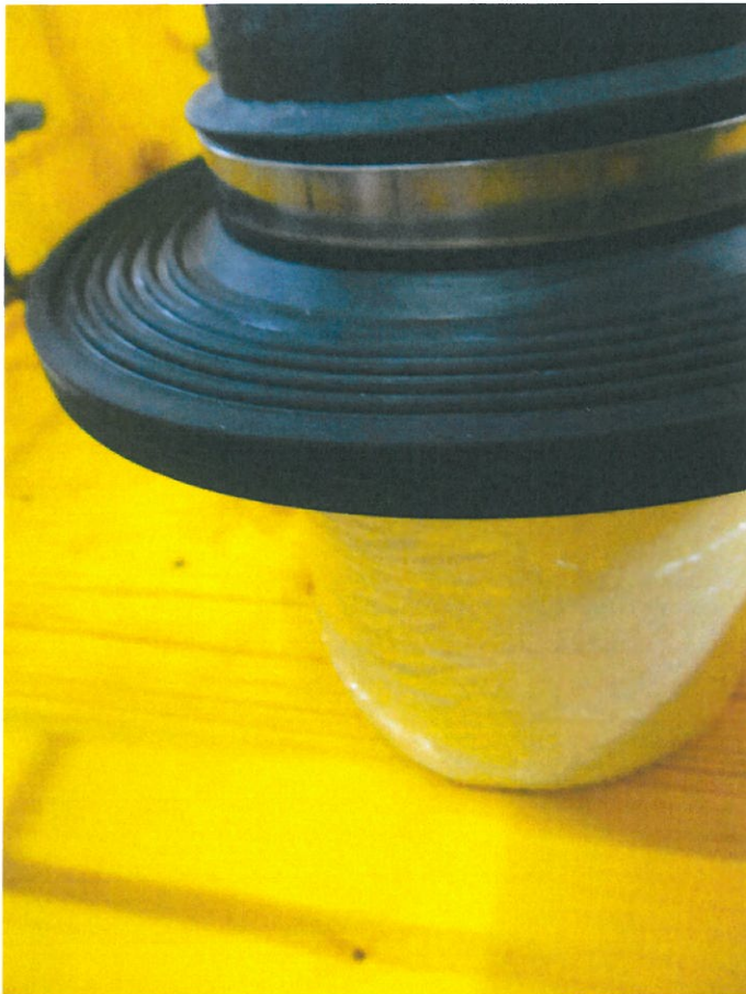
Figure 3: The PE pipe encased with fleece fabric on one side to guarantee that water is transported to the pipe collar
